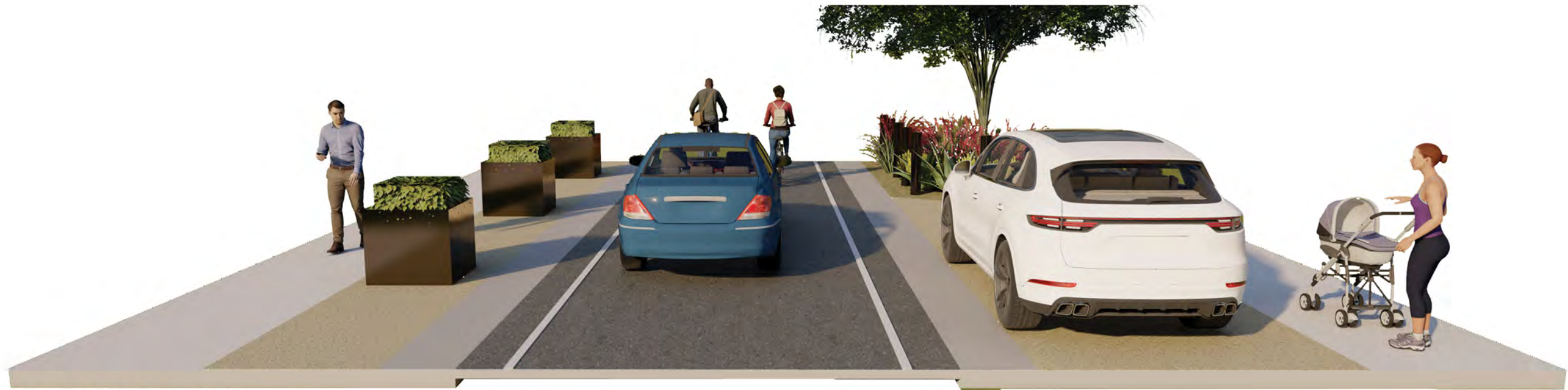
Proposed Section @ 16-ft wide clearance
